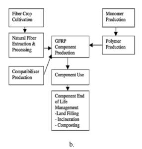
Figure 14(a). Lifecycle of a glass fibre-reinforced composite component. (b) Lifecycle of a natural fibre-reinforced composite component (Joshi et al., 2004)
