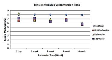
Figure 7. Tensile Modulus (GPa) at different environmental conditions (Ghani et al., 2012)
