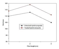
Figure 3. Hardness of the untreated and treated epoxy-based sisal-glass hybrid composites with different fibre lengths (Ashok et al., 20102)
