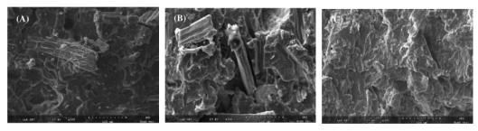
Figure 10. The cross-sectional micrographs of the extruded PLA pellets with different reinforcement loadings: (A) kenaf 30 wt%, (B) kenaf 15 wt% and corn husk 15 wt%, and (C) corn husk 30 wt% (Kwon et al., 2014)
